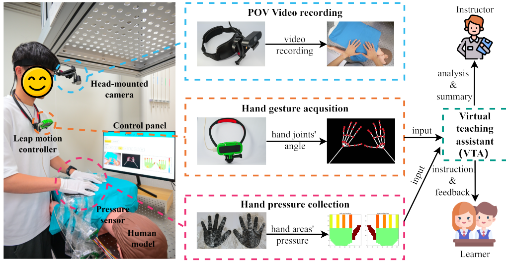
Figure 2: The Multi-modal Remote Learning System for Massage Consists of Four Major Components: 1) POV Video Recording: records the instructions and learners' performance; 2) Hand gesture acquisition: collects the gesture data (joints' coordinates); 3) Hand pressure collection: collects hand pressure data from six areas of each hand (five fingers and palm); 4) VTA: provides real-time review to the learners and learners' summaries to the instructors.
